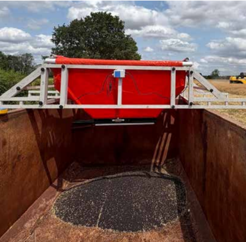
A bag weigher used for WOSR Pioneer Accurate Crop Testing System (PACTS ® ) trials. Combine discharges are weighed using the electronic console, a grain sample is taken for moisture and oil analysis, and the grain is then released from the bag into the trailer.
